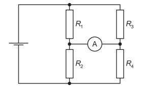
The four resistors have different resistances  $R_1$ ,  $R_2$ ,  $R_3$  and  $R_4$ .
